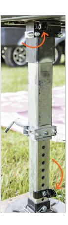
**NOTE:** The lower bracket bolt should go into the same hole that holds the landing leg foot. If this is not possible, then bolt it onto the first available hole above the foot.
