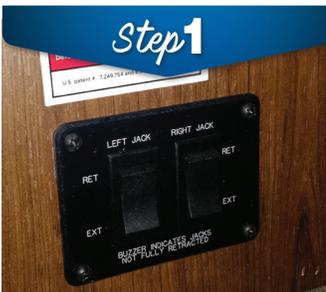
Use the extend and retract buttons in the coach to extend or retract the stabilizer legs. The arms operate and are controlled independently of one another.
