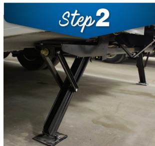
**TO EXTEND:** Press the “EXT” buttons until each leg reaches the ground. The sound of the motor will change pitch as the legs begin to take weight. Adjust each side independently for desired stability.
