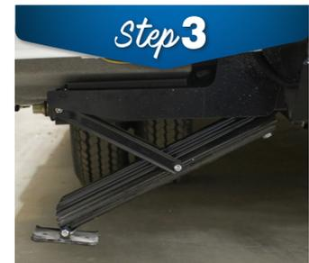
**TO RETRACT:** Press the “RET” buttons simultaneously until each leg is fully retracted.
