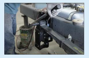
NOTE: The kit may include a jounce bumper plate. If so, install the bolts and tighten and torque to 40 ft-lbs.
