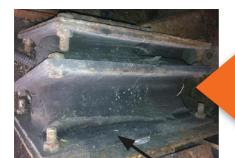
Tears exceed 3" long and 3/4" deep, springs SHOULD be replaced.
