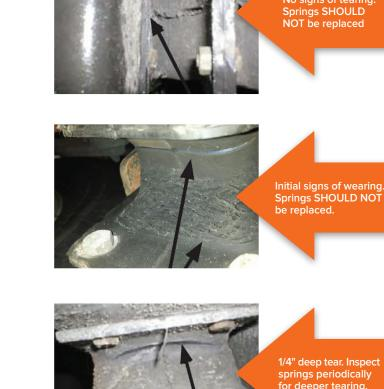
1/4" deep tear. Inspect springs periodically for deeper tearing.
