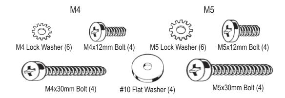
Hardware for securing bracket: Select the appropriate length based on the thickness of your mounting surface.
