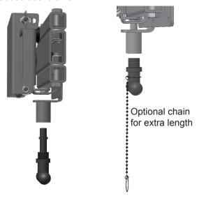
STEP 2 Secure the wall bracket to mounting surface: Pre-drill holes using a 1/8" drill bit for use with 1/4" lag screw. Use 1/4" bolt (not included) or lag screws.
