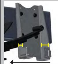
**NOTE:** There may be left side and right side frame hangers. If so, the narrower, smaller cap gusset will always face forward to provide leaf spring clearance.
