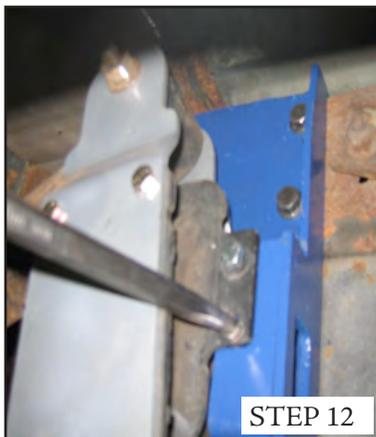
**STEP 12** Using a drift pin align the back bottom rubber spring mounting hole to the frame hanger mounting hole. Install the provided 7/16 x 1 1/4-14 bolt in the hole above the drift pin. Repeat this procedure on the opposite side. Raising the axle may help to align the remaining holes. Install the remaining rubber spring mounting bolts and torque to the appropriate specification. Torque the leaf spring eye bolt to 40 ft lbs.
