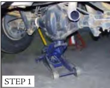
**STEP 1** Be sure to block the front tires. Place floor jack under the differential and raise drive axle tires a minimum of 12" off the ground.
