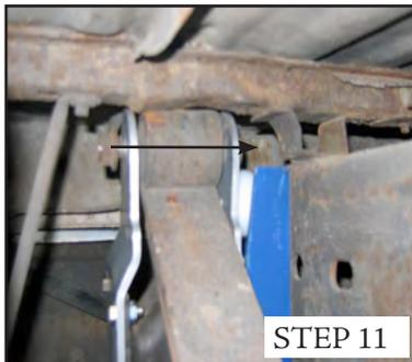
**STEP 11** Use the floor jack to raise the axle until the rear spring eye is above the OEM frame rail. Using the spring eye bolt, install the spring carrier assembly onto the leaf spring. \*The bolt head must face towards the OEM frame rail.
