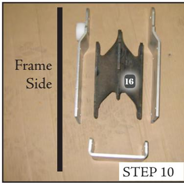
**STEP 10** Note the orientation of the rubber shear spring assembly, spring carrier, spring carrier with plastic disk, and the jounce bumper bracket. The spring hanger with the plastic disk will be positioned against the frame hanger. Install the rubber spring so the side with identification number is attached to the spring carrier without the plastic disc.
