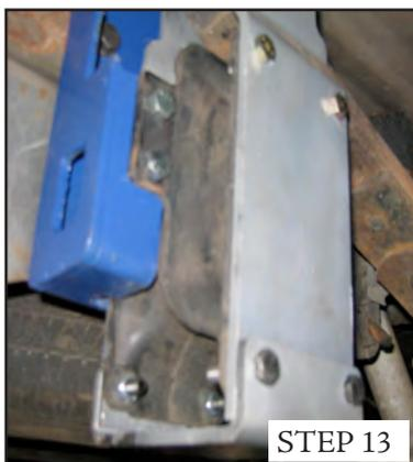
**STEP 13** Perform final check. Be sure all nuts and bolts are properly torqued. Refer to torque chart on Page 2. Verify the spring eye bolt is positioned with the bolt head toward the frame.
