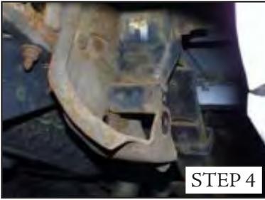
**STEP 4** To facilitate installation one may want to remove the spare tire. Remove the rear spring eye shackle nut and bolt. If possible, raise the drive axle and remove the shackle nut and bolt over the top of the frame. If the spring hanger is above the leaf spring eye, lower the leaf spring to remove the spring eye bolt.
