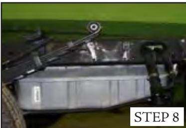
**STEP 8** The frame and leaf spring are now ready for installation of the MOR/ryde components.
