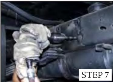
**STEP 7** With the appropriate drill bit, ream the existing spring hanger hole to be sure that the hole is clear of any debris. These holes will be used to bolt the MOR/ryde frame hanger to the OEM chassis.
