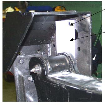
There is an Allen head bolt at the top to be removed. Hold the nut with a ½" end wrench.
