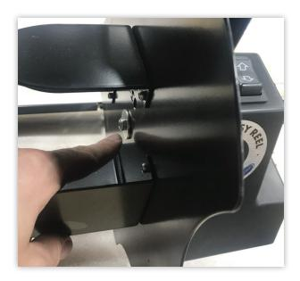
3. To check the gearbox, remove the motor cover (3 bolts) then remove the motor bracket (2 bolts) at this point apply power to the motor, if the motor is turning but the
