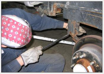
Wet Bolt 2.90" long (h) and fasten with one 7/16"-20 Flange Lock Nut (e). Tighten with 13/16 socket and wrench, torque rating
