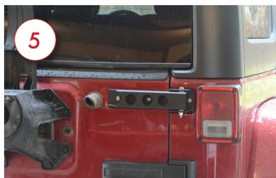
**NOTE:** The hinge includes a grease zerk, we recommend greasing the hinges on initial installation and thereafter greasing the hinges whenever the chassis or other body mounts are greased.
