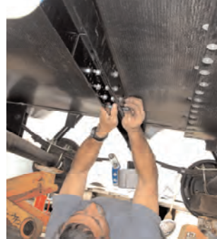
Follow the bolt pattern listed in the instruction manual for the crossmember. Torque to spec once it's in place.
