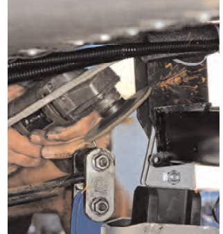
For our installation, we had to grind notches in the spring hanger in order for the crossmember bolts to fit properly.
