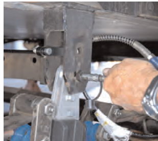
Before installing the tires, grease all bolts with zerk fittings with a high-pressure grease gun.
