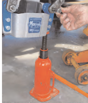
Use a hydraulic bottle jack to raise or lower the SRE to properly align the bolt holes.
