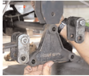
Once the equalizer is removed, discard the upper bolt and save the links for the SRE install.
