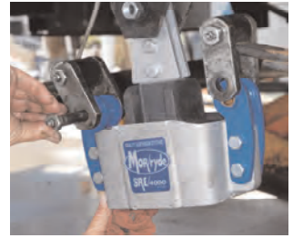
Install the new SRE equalizer with the new upper bolt and existing links (replace if worn); grease bolts prior to insertion.
