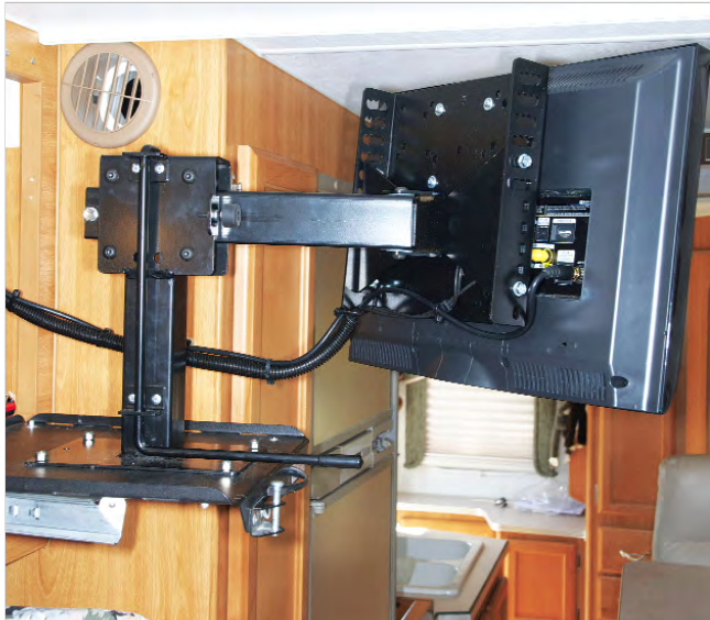
With the sliding arm fully extended, the TV can be rotated for viewing from just about any location in the camper. A small hole was cut in the bracket to allow access to the connecting cables.
