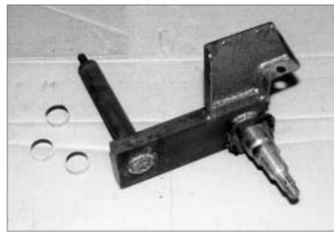
A single suspension trailing arm element shows the three fiberglass collar bearings (left), the stub axle on which the trailing arm pivots, the wheel spindle and the metal bracket to which the springs and shock are attached.
