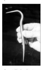
A special brake-adjusting tool with a sharply bent end, available at auto-parts stores everywhere, is required to reach the brake adjustment point on the new axles.
