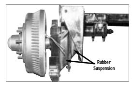
Diagonal-shaped parts to the right of center (arrows) are the rubber suspension block elements. The shock absorber is not installed in this view.
