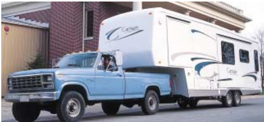
The RE System was tested on a 29-foot Carriage Cameo LXI fifth-wheel trailer, towed by a Ford F-250 pickup. The test route covered ten miles of broken pavement, rough asphalt and other poor road conditions.
