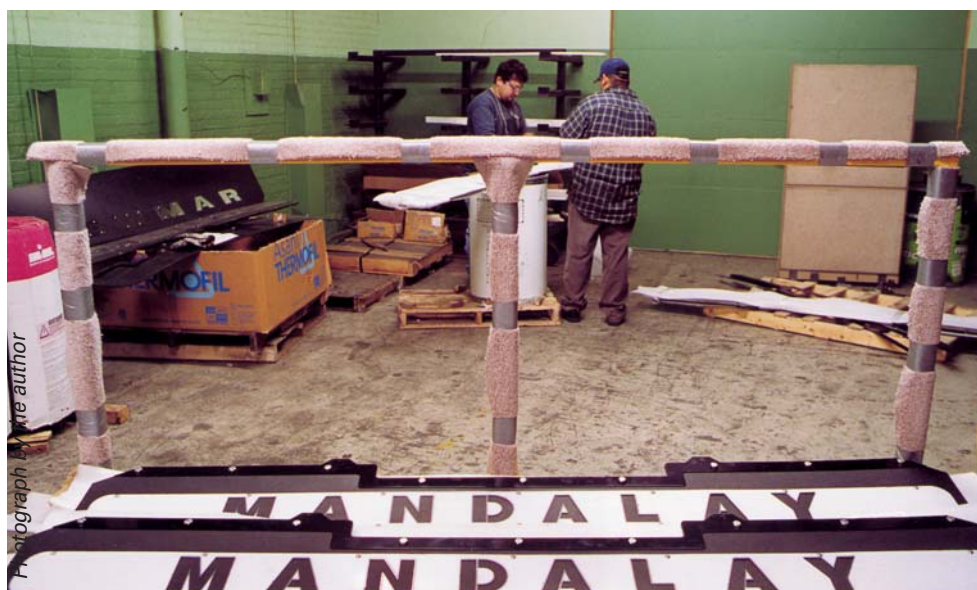
Monogrammed RV mud guards are one of the new products made possible by the MVP lasers. The guard is a strip of 0.080-in. polished 304 stainless steel bolted to a ribbed rubber flap.
