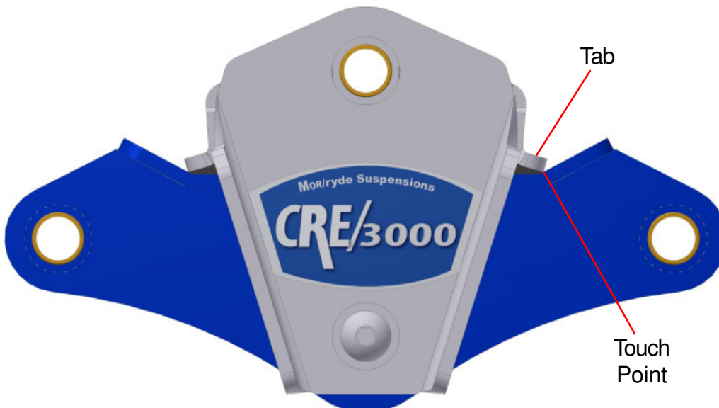
CRE/3000 with rubber spring worn out shown at design load. Note: Tabs must touch on BOTH sides of beam arm for rubber to be worn out.
